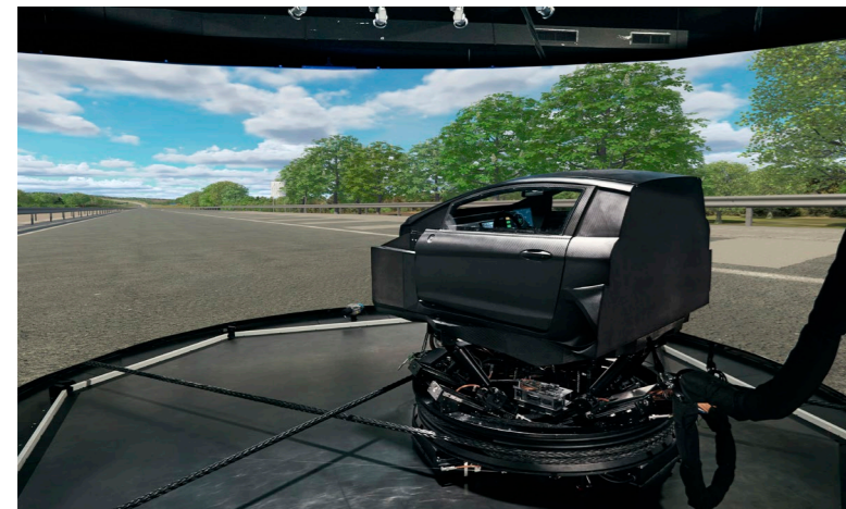
DiM FSS Hyperdock is a highly optimised carbon-fibre cockpit delivering higher frequency vibration, part sound for an integrated experience
